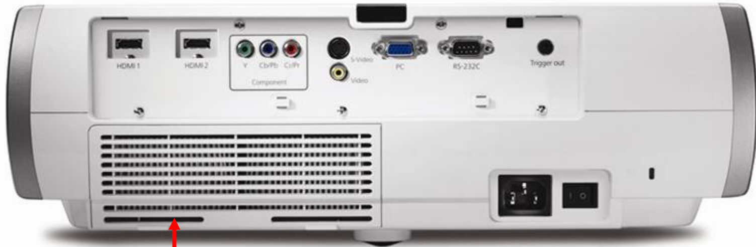
Dust filtration system
